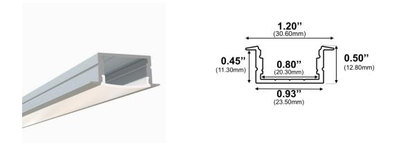
The CH-L25P91 is a specialty low profile designed for recess flush fit into any surface. Perfectly designed to be used as a main light source.
